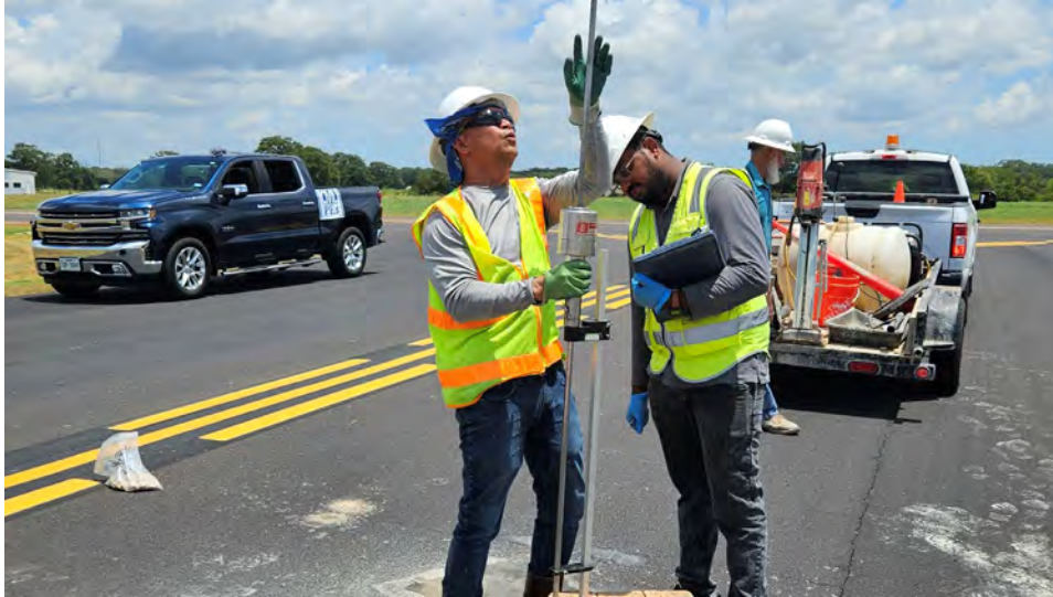
Figure 2 - DCP Field Testing
