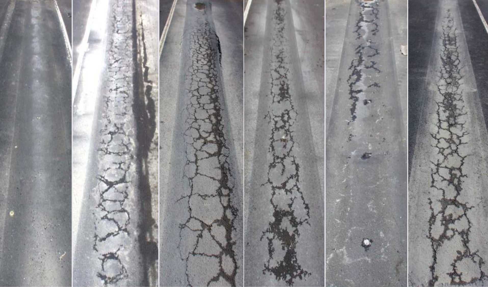
Lane 1 Lane 2 Lane 3 Lane 4 Lane 5 Lane 6 CR-AZ Control Air Blown SBS LG CR-TB TP 300,000 100,000 100,000 300,000 100,000 200,000
