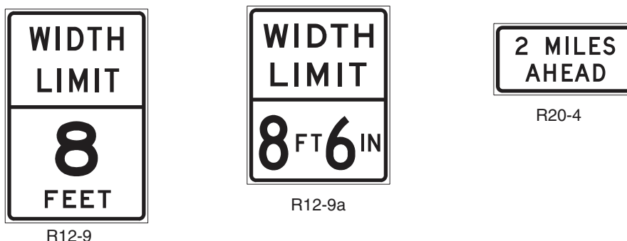
Figure 2B-20A. Width Limit Signs
